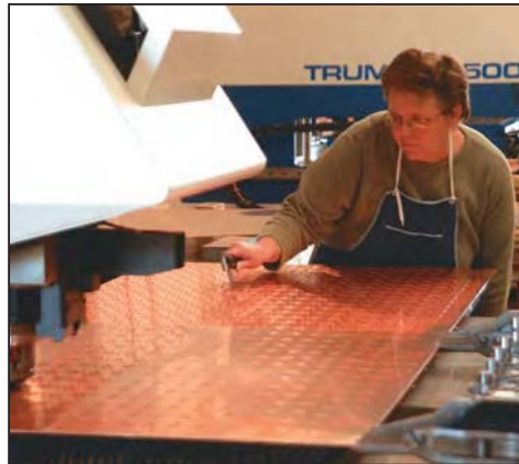
Custom shapes and sizes are produced quickly and accurately on our Trumph Punching Machines.
